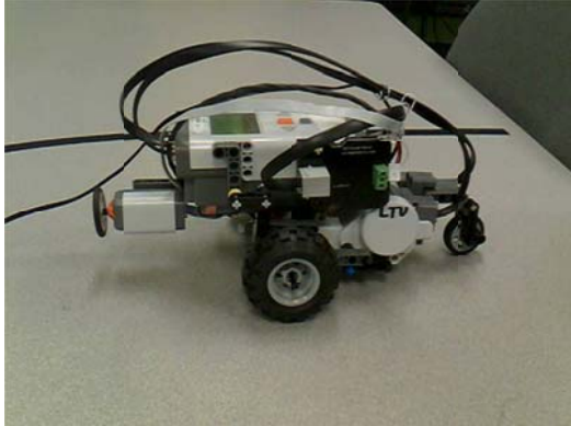
Robot A: Rear swivel wheel.
