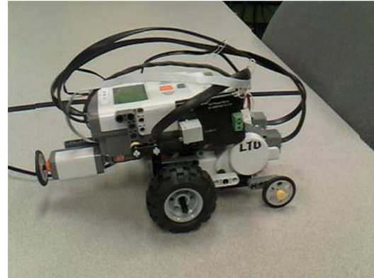
Robot B: Rear non-swivel wheels.
